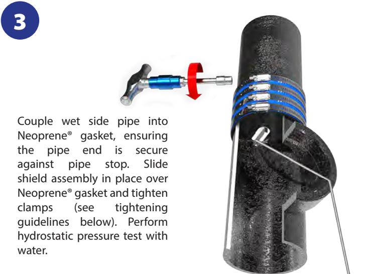
Couple wet side pipe into Neoprene® gasket, ensuring the pipe end is secure against pipe stop. Slide shield assembly in place over Neoprene® gasket and tighten clamps (see tightening guidelines below). Perform hydrostatic pressure test with water.
